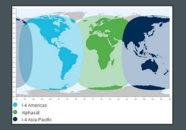
Network of satellites covering the entire globe, with the exception of the north and south poles IsatPhone 2, was created for remote regions in which conventional cell phones do not operate, such as plantations, forests and ocean. The device is portable and robust, being able to be used in the most diverse environments and under extreme climatic conditions as long as it is aimed towards the sky.
